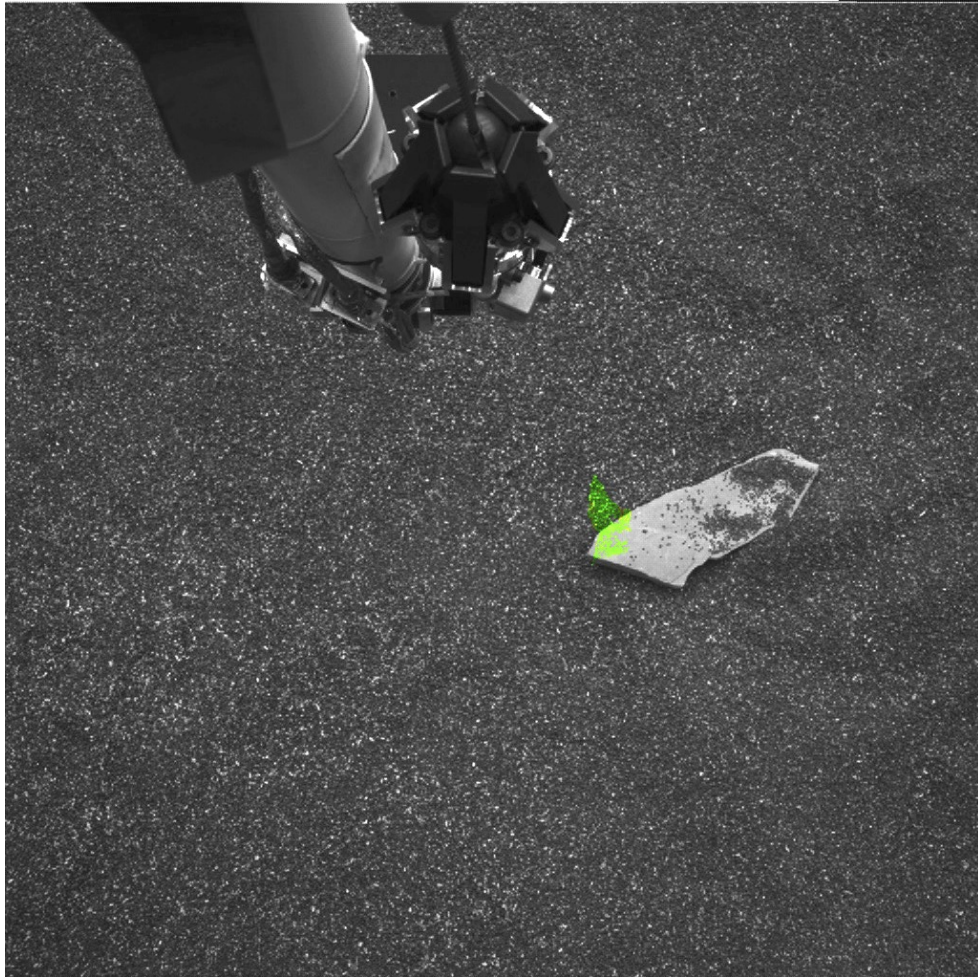
Figure 5-13: Instrument Delta Tilt for SEIS/WTS (TDS) Data Overlaid onto Image EDR. Green indicates good (state=5).
